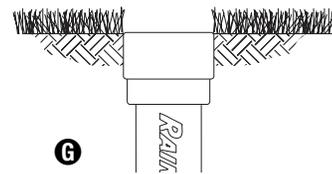
**NOTE:** To remove sod cup you must first unscrew the internal from the outer rotor case. Then you must remove the inner cup by unlatching the retainer clip. Then you can take the outer cup off of the rotor collar.
